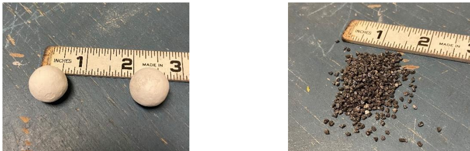
Figure 4. Corundum material used to patch cathode blocks. Left: spheres, Right: grains.
